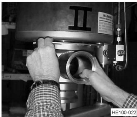
**Figure 48 - Close Locking Latch**
