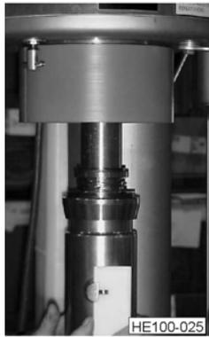
**Figure 47 - Blade Alignment Tool Installed**
