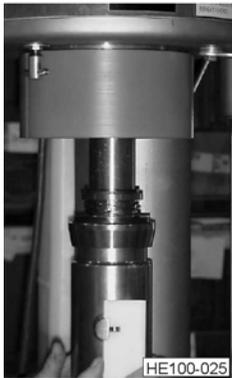
**Figure 71 - Exposing Top Mechanical Seal**
