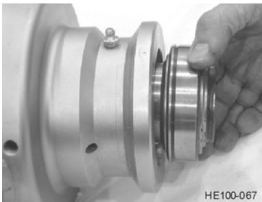
**Figure 23 - Lubrication Ring Orientation**
