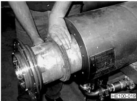
**Figure 40 - Tube Removal**
