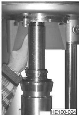
**Figure 46 - Align One Half of Blade Alignment Tool**
