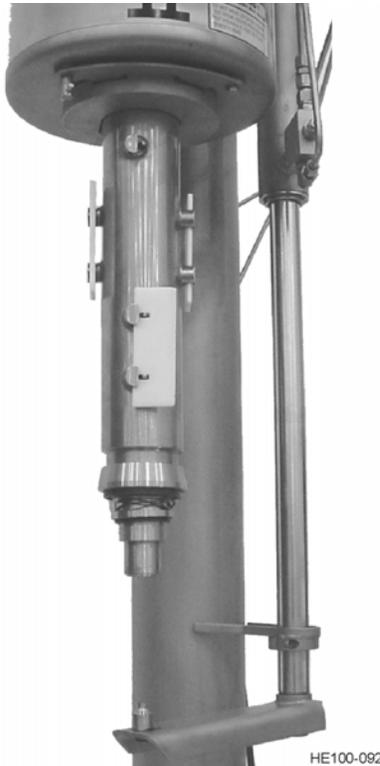
**Figure 75 - Shaft With Head Removed**
