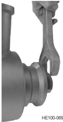
**Figure 37 - Installation of Shaft Lock-nut**
