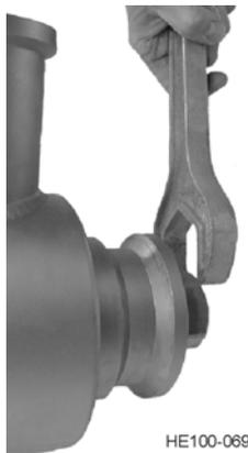
**Figure 27 - Removal of Shaft Locknut**
