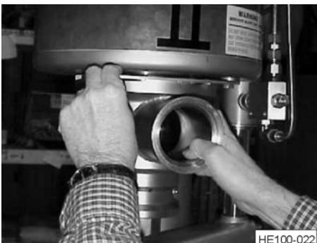
**Figure 43 - Disengaging Locking Latch**
