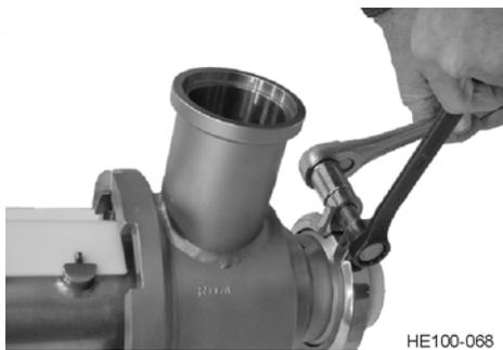
**Figure 38 - Installation of Hinged Clamp**
