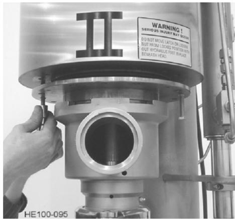
**Figure 51 - Insert Jack Screws**
