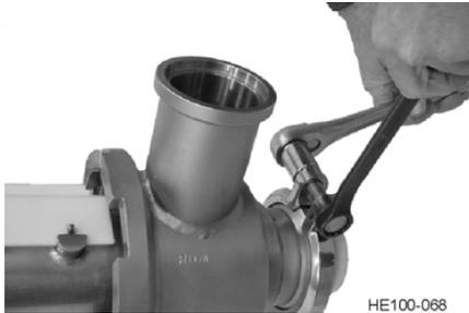
**Figure 26 - Removal of Hinged Clamp**
