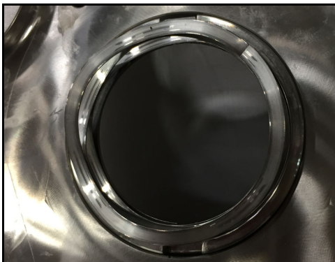
Figure 59 - Wave spring installed
