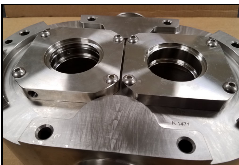
Figure 162 - Seal housings installed
