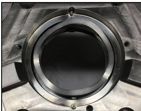
Figure 96 - Wave spring installed
