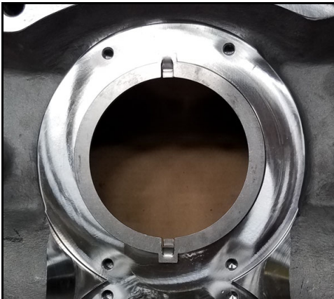
Figure 64 - Drive ring installed
