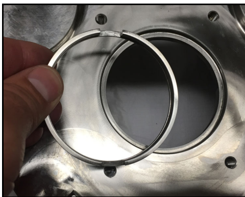
Figure 54 - Install shaft ring
