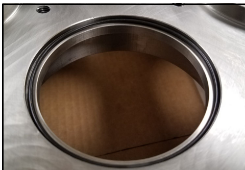
Figure 158 - Seal housing O-ring installed
