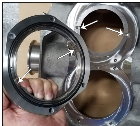
Figure 113 - Seal housing O-ring installed
