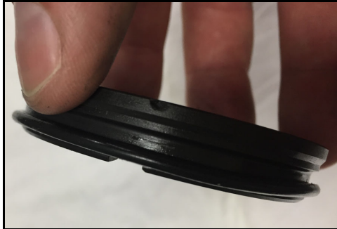
Figure 134 - Seal O-ring installed
