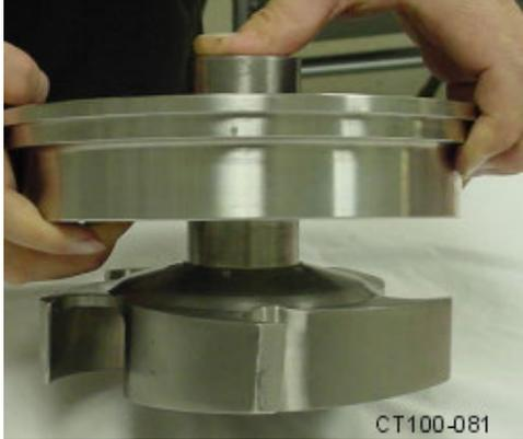
**Figure 37 - Move Rotary Seal Up Shaft**
