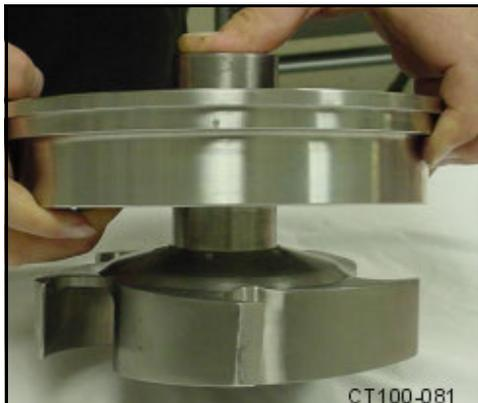
**Figure 25 - Moving Rotary Seal Up the Shaft**
